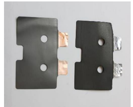
Figure 1. Copper anode and aluminium cathode foils coated with lithium ion compound demand high cutting speed and near perfect edge quality to replace punch press machines and render components that can be tightly packed without electrical leakage.
