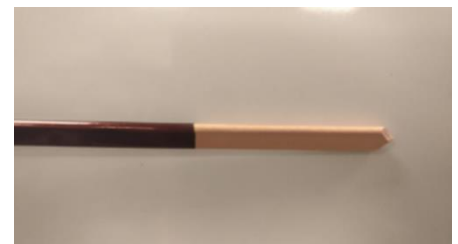
Figure 4. Hairpin ablation of dielectric coating prior to welding using ns pulsed fiber lasers offers a cleaner, faster and more repeatable result that wire brush mechanical removal.
