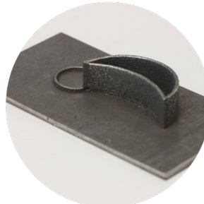
Cladding Dissimilar Metals
