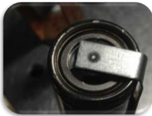
Battery Cell Al on Ni-Steel
