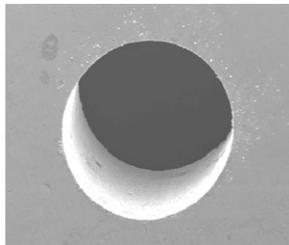
0.5mm thick 304SS; 50 $\mu$ m dia
