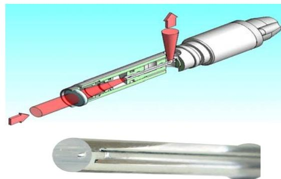
Figure 3: PIPA fiber delivery termination
