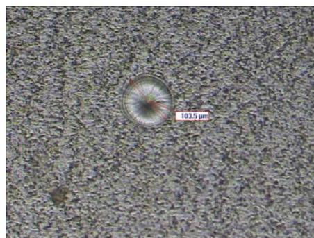
30+30+200µm 304SS; weld dia 104µm
