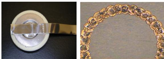
Cu/Al spot welds; Cu battery terminal spot welded
