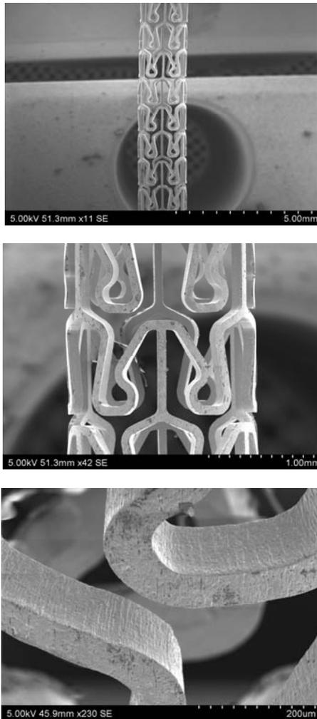
Figure 8: 316SS, nitrogen assist gas, 10µm spot size; modulated output
