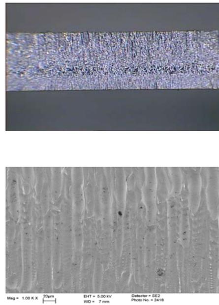
Figure 9: SM fiber cut; 1.8 mm thick wafer, 10 kHz, 350W, >3.5m/min; nitrogen assist gas
