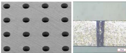
1.5mm thick nickel based alloy; 150 $\mu$ m dia
