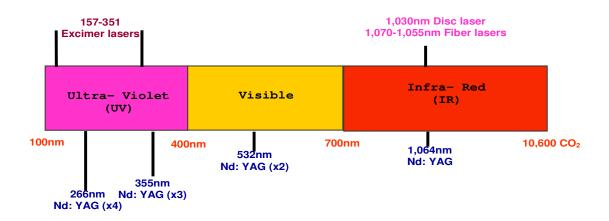
Figure 1: Some of the laser sources for micromachining applications
