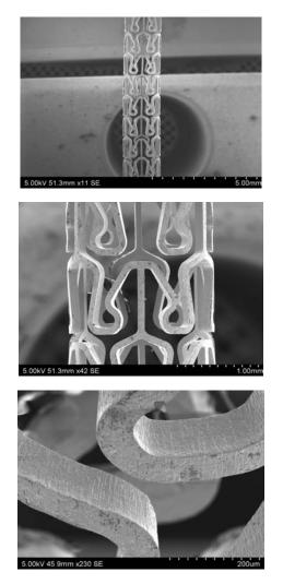
Figure 8: 316SS, nitrogen assist gas, 10µm spot size; modulated output
