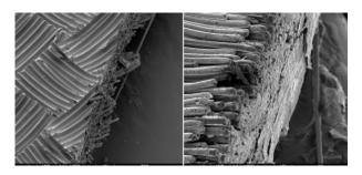
Figure 11: SEM image on the left, mechanical cut 500X. SEM image on the right fibre laser cut 1200X
