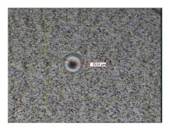
30+200µm 304SS; weld dia 76µm
