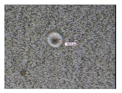
30+30+200µm 304SS; weld dia 104µm
