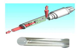
Figure 3: PIPA fiber delivery termination
