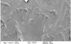
Figure 10: Pulsed laser cut; 2.0 mm thick wafer, .>0.15m/min; nitrogen assist gas
