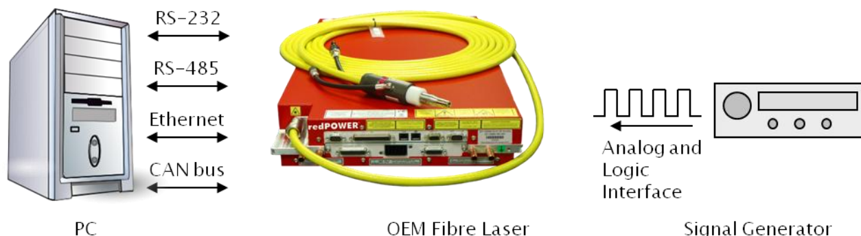
Figure 1 Control Connections to OEM Fibre Laser
