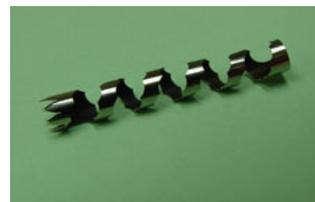
Figure 7: Nitinol tube (nickel- titanium alloy); 50W fiber laser; modulated output, spot size 12 $\mu$ m, argon assist gas
