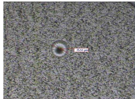
30+200µm 304SS; weld dia 76µm
