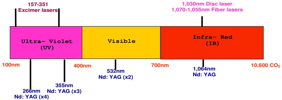
Figure 1: Some of the laser sources for micromachining applications
