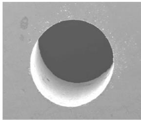
0.5mm thick 304SS; 50 $\mu$ m dia
