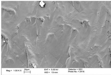
Figure 10: Pulsed laser cut; 2.0 mm thick wafer,  $>0.15\text{m/min}$ ; nitrogen assist gas
