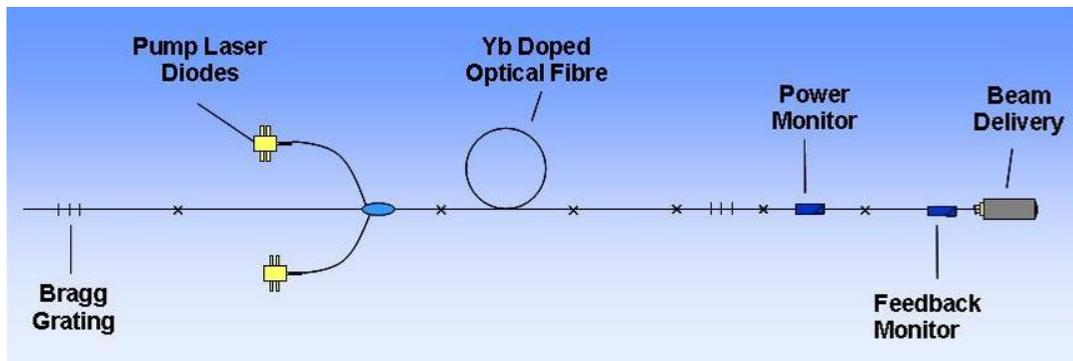
Figure 2: Schematic diagram of single mode fiber laser
