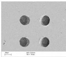
0.6mm thick alumina ceramic; 50 $\mu$ m dia
